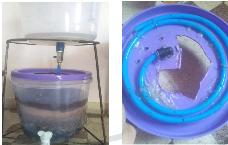
Figure: Filtration and sprinkler setup
