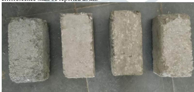
Fig 5.4 After efflorescence test
