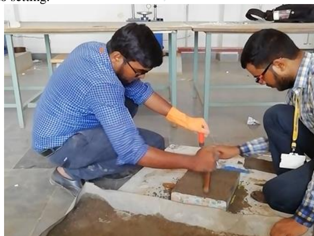
Fig 4.2.1: Placing by compacting
