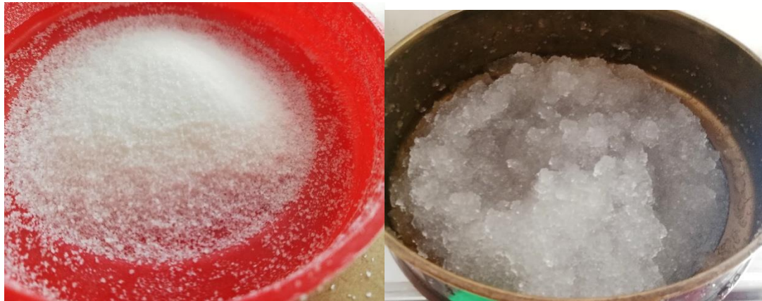
Figure 1 Sodium polyacrylate before and after absorbing water
