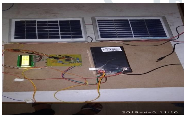
Fig3., Battery Charging on Solar Panel
