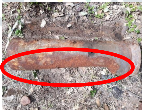
Figure 16: Wear of roller axle
