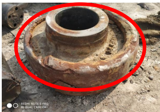
Figure 11: Wear of track wheels on periphery
