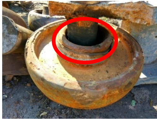
Figure 13: Wear of bushes
