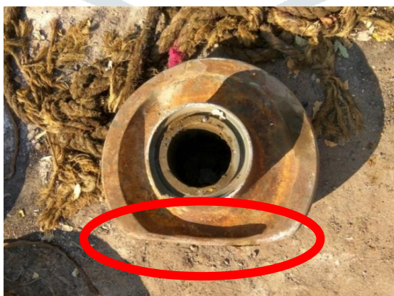
Figure 12: Flattening of the periphery
