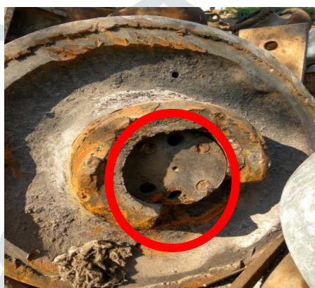
Figure 15: Lock plate bolt shear or missing
