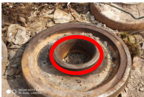
Figure 14: Wear of track wheel bore
