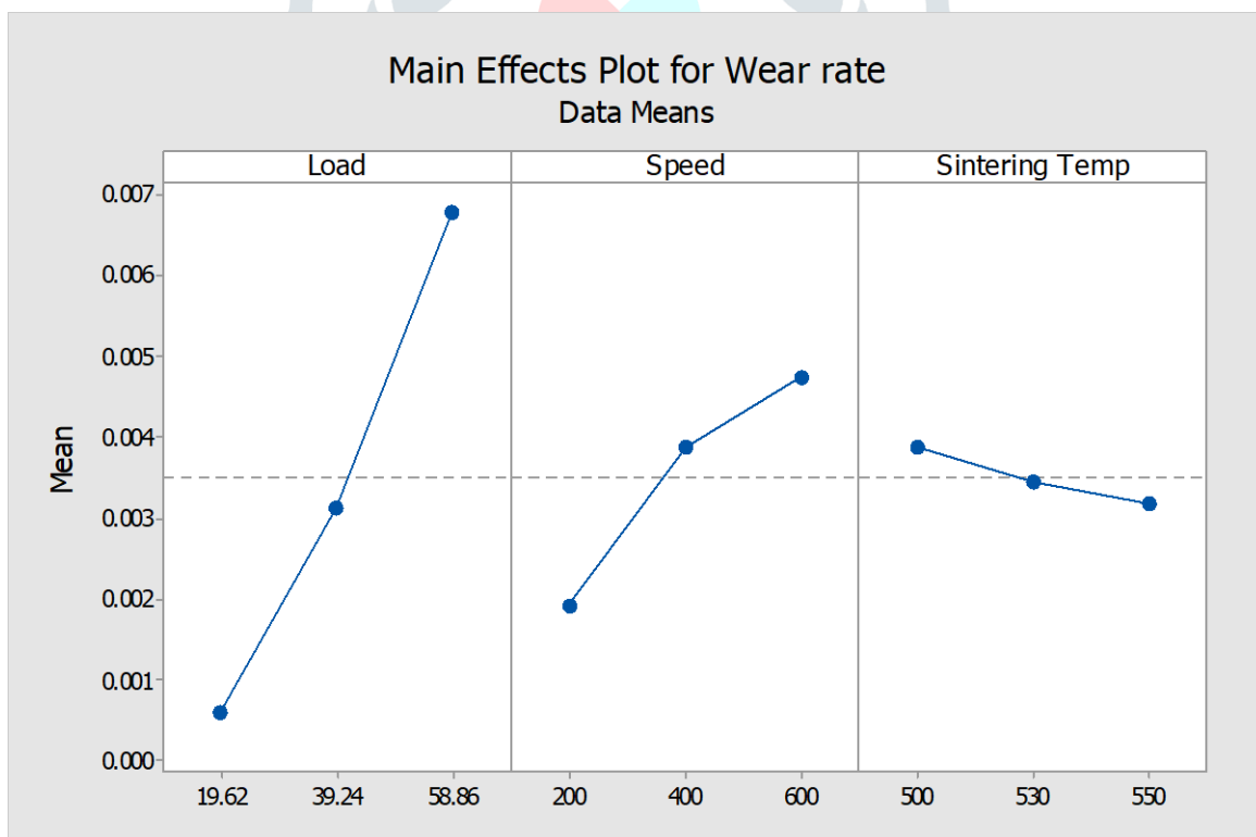
Figure 2: Main Effects Plot for mean of Wear rate
