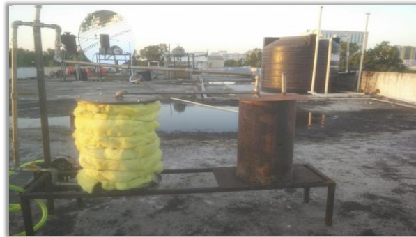
Figure 1. The experimental setup of the flat plate solar collector for solar thermal storage system
