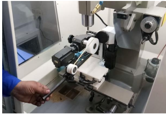
Fig - 8 Attaching collet in CNC machine
