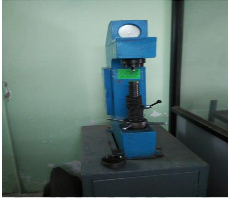
Fig 2: Dial gauge operated brinell hardness tester machine
