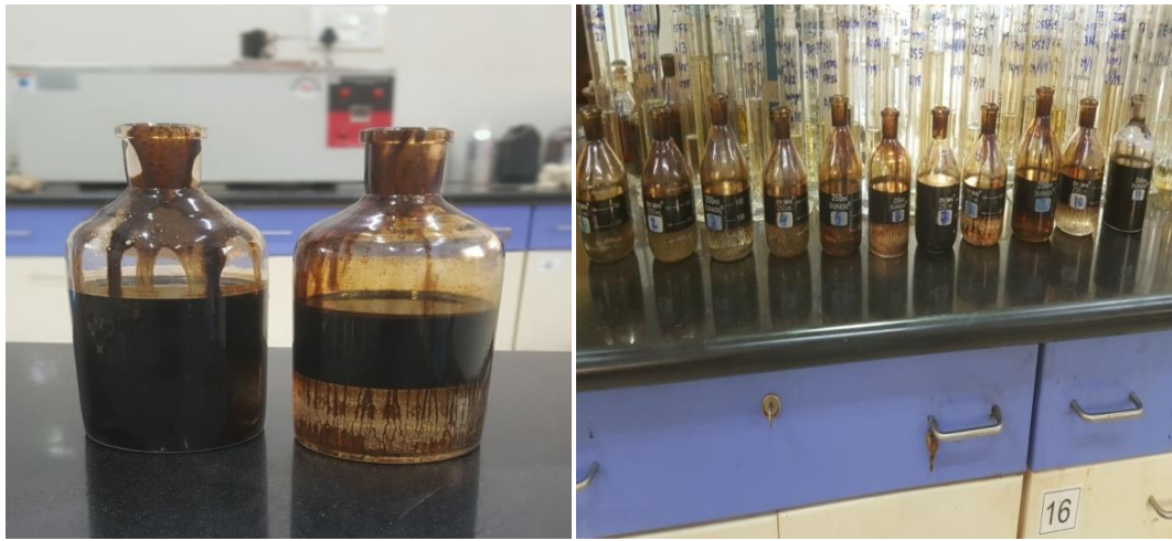
Fig 4: Separation of water after Demulsification
