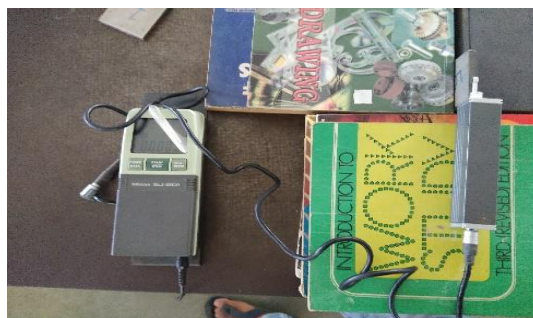
Figure 4. Surface roughness tester (Mitutoyo SJ210, Taylor Hobson)
