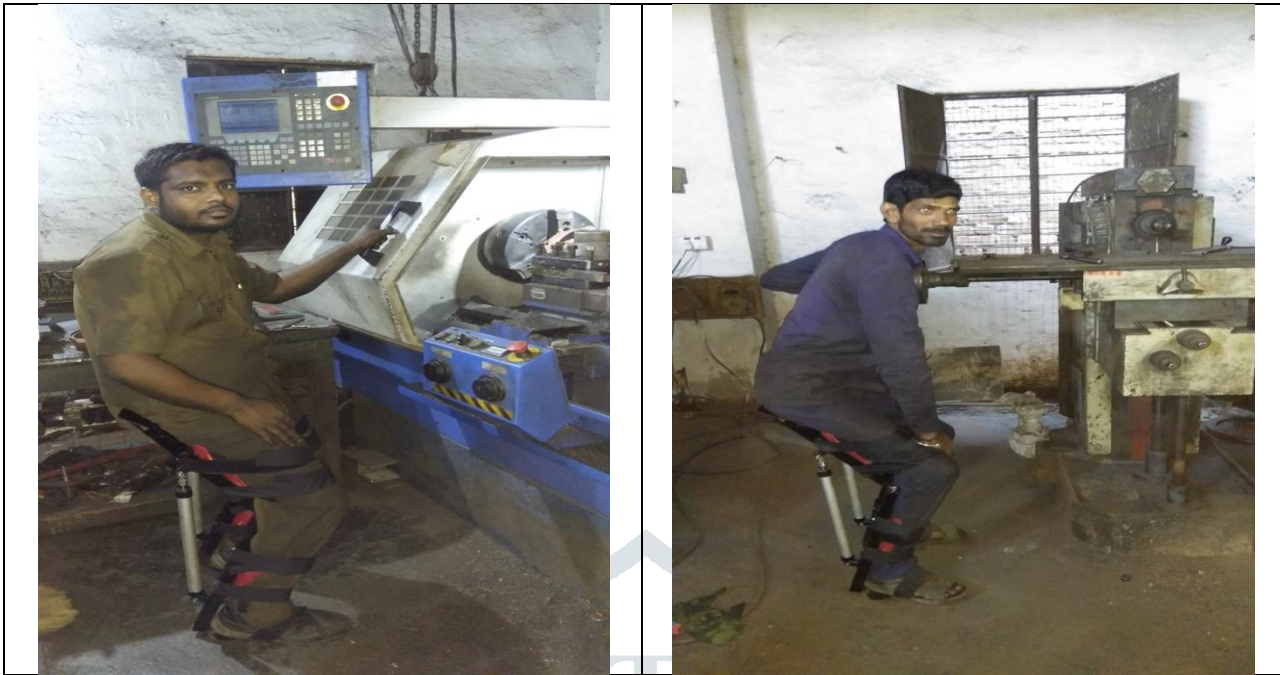
Fig.2 Actual use of Wearable Chair at Workplace
