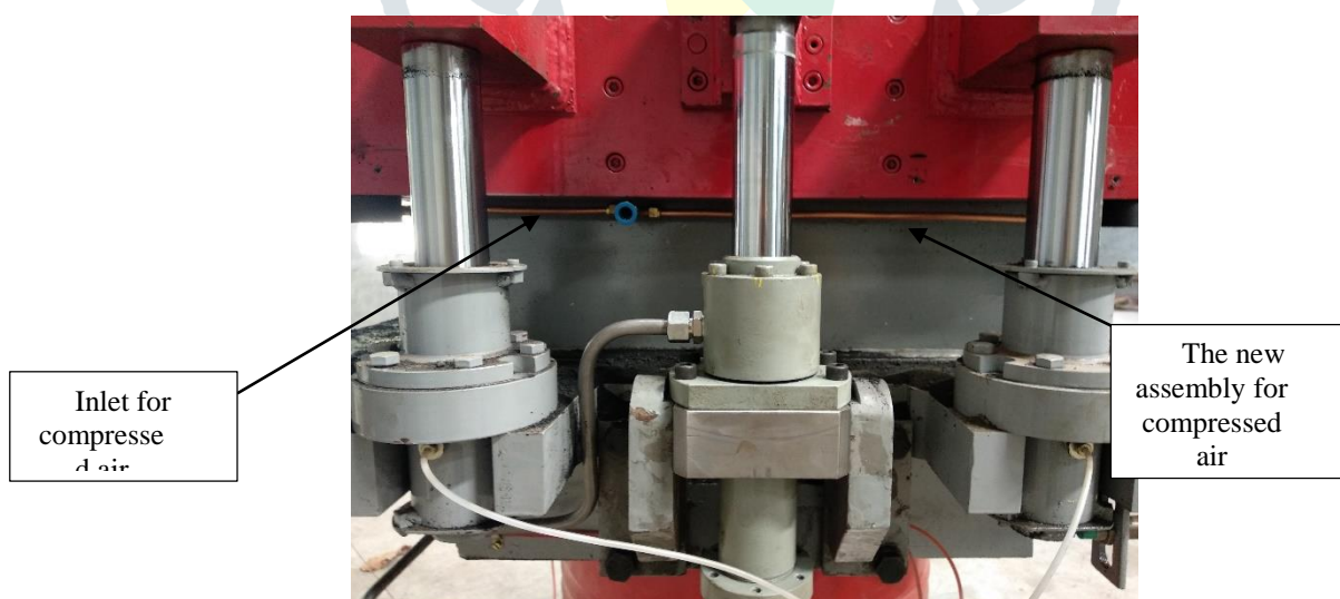
Figure 8: copper tube assembly for compressed air.
