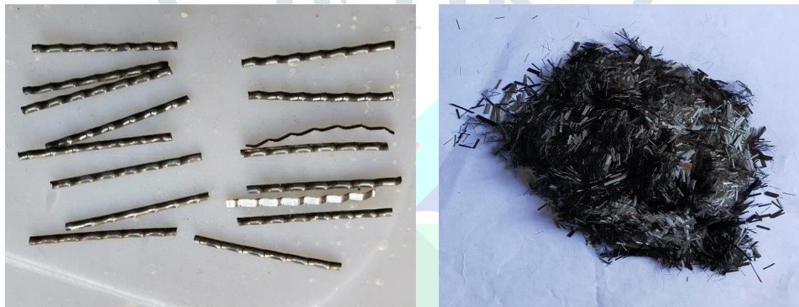
Fig. 1: Steel Fibers and Chopped Carbon Fiber
