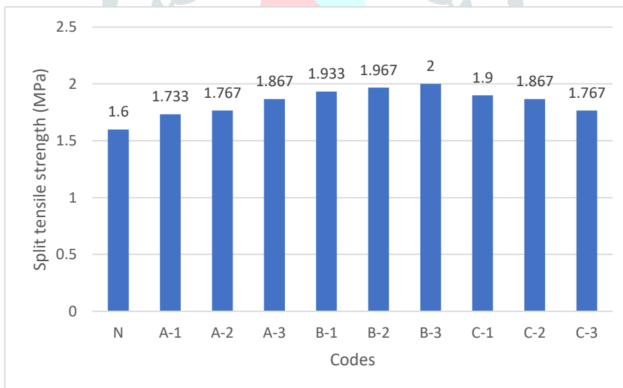
Fig. 4: 7-Days Split-Tensile Strength
