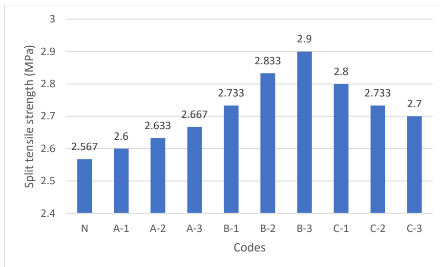
Fig. 5: 28-Days Split-Tensile Strength
