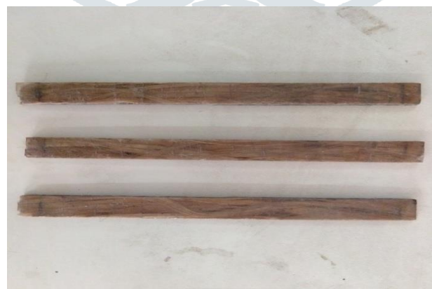
Figure 5: 30% jute 20% sisal and 50% epoxy resin composition
