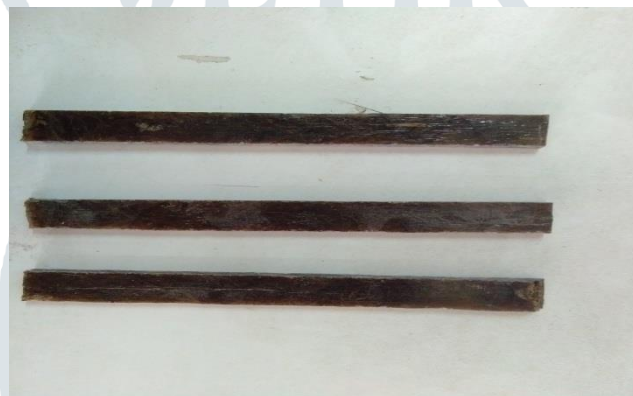
Figure 4: 20% jute 30% sisal and 50% epoxy resin composition
