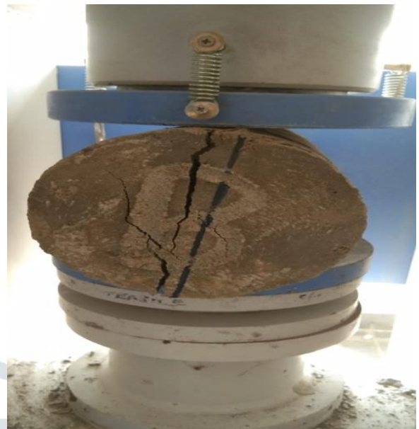
Fig.3: Test Setup to check split tensile strength of cylinder
