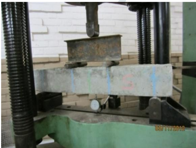
Fig.2: Test setup to check flexural strength of beam
