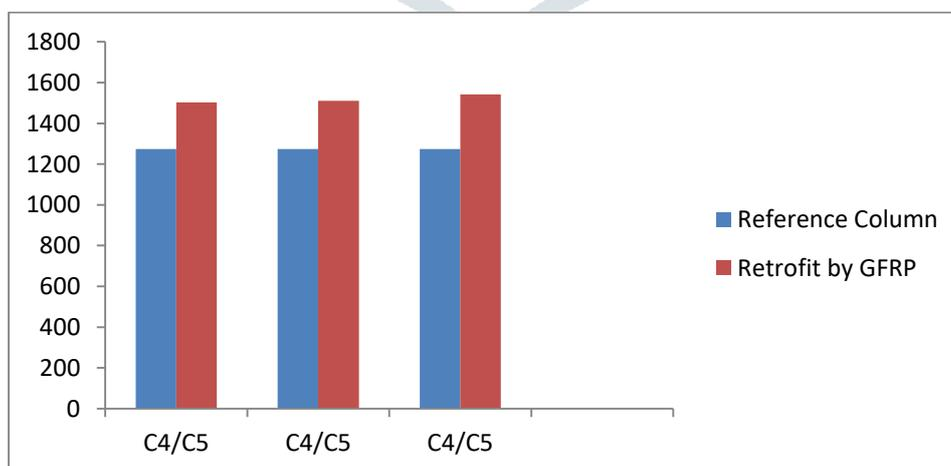
**Chart-1 Comparison between Reference Column and Retrofitted by GFRP**
