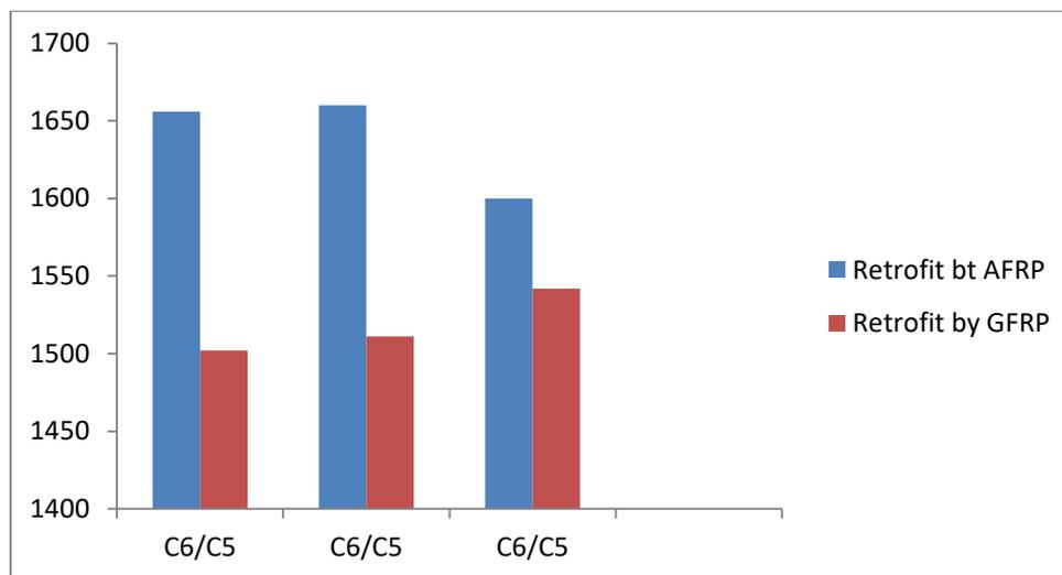
Chart-3 Comparison between Retrofitted by Aramid and Retrofitted by Glass
