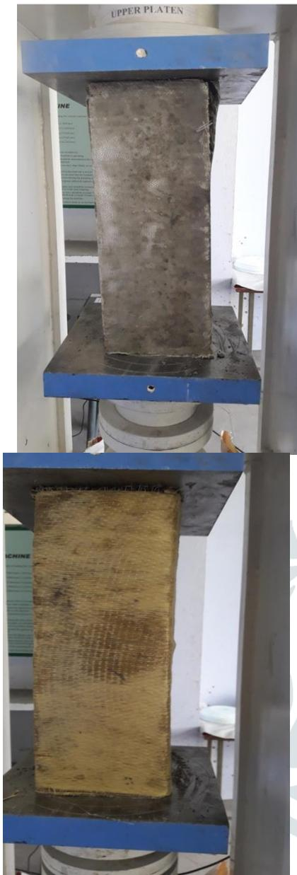
Fig - 5 Aramid fiber wrapping (AFRP)
