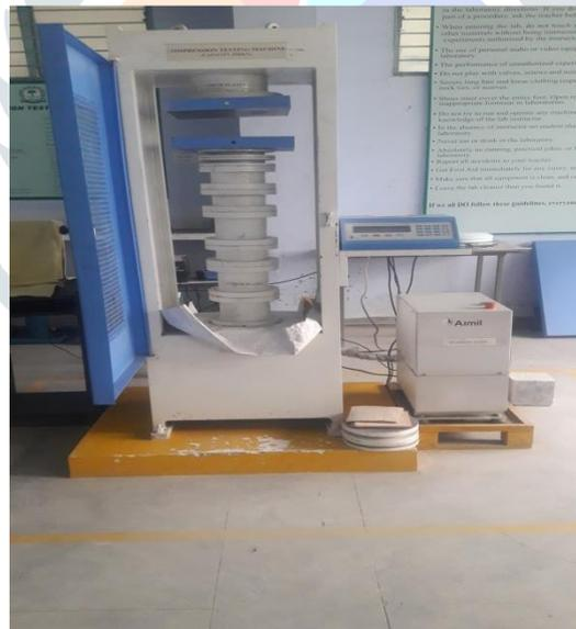
Fig.- 4 Compression Testing Machine
