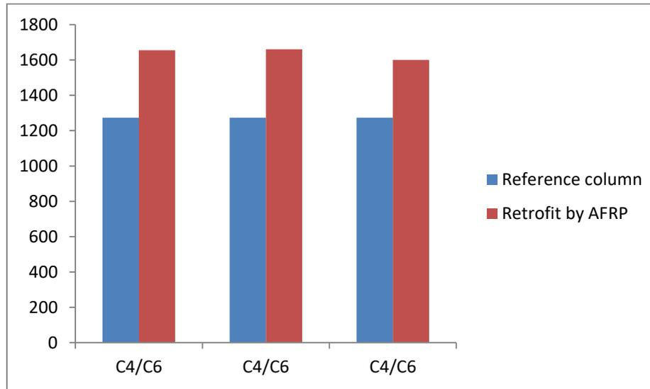
**Chart-2 Comparison between Reference Column and Retrofitted by AFRP****Table 4.4 Comparison between Retrofitted by Aramid and Retrofitted by Glass**
