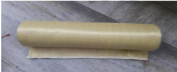
Fig. 1 Aramid Fiber Fabric
