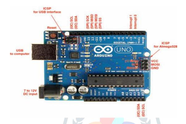
First choice for this development of side stand will be arduino 328 microcontroller because arduino microcontroller don't need external programming sources because it has capacity for internal programming by itself so it's automatically utilise the program by itself and it support any advanced operating system like windows, McIntosh so there is no problem for programming for theproposed circuit.
