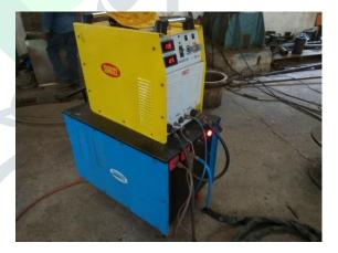
When current is 90A arc is very small very unstable and heat input is very slow so it take more time to weld the plate and finishing is not good as compare to 140A. In this experiment same current at each layer means suppose in the first experiment root &
