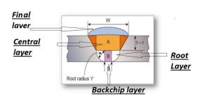
"A" = final finishing layer "B" = central layer filler layer" "C" = Root Layer base layer
