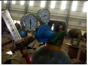
In next 18 - 24 experiment having Gas Flow Rate is 15 LPM, current variation 90A-140A with increment in 5A current at each layer of weld which is describe in experimental methodology.
