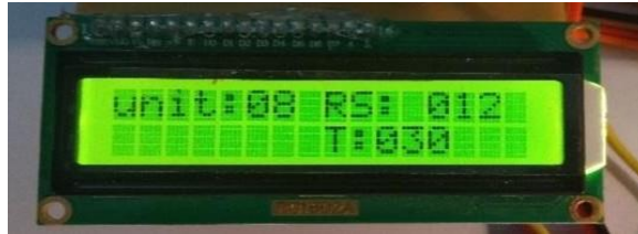
Fig.3. LCD display that represents the consumed units, rupees and temperature
