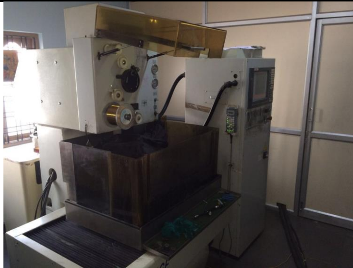
Figure 2: Wire EDM machine on which the work piece was machined
