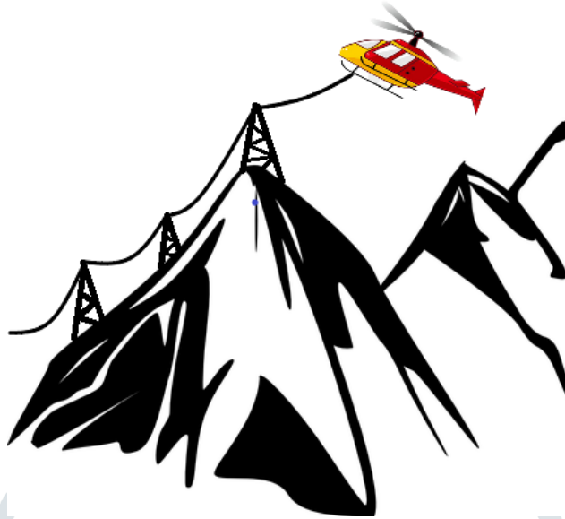
Figure 2 Stringing using Helicopter in Hilly area.
