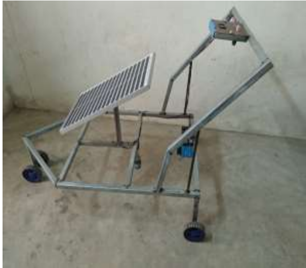
Fig. fabrication of solar grass cutter
