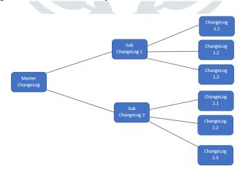
The following code block shows how we have refactored the original changelog file for our liquibase database as it can be seen, we have *included* reference to different XML files. Each changelog will run in order when liquibase starts running.
