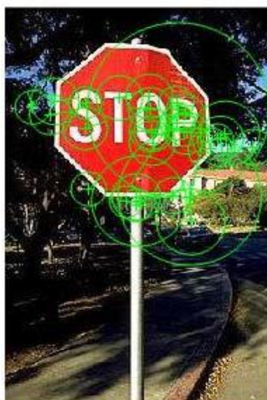
Fig 5 : SURF feature detection in features points matching Stop sign image
