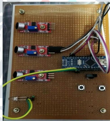
Figure 3 image of the voice modulation circuit
