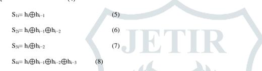
Where  $i, j \in [1, n], i \neq j$ . Equations (4)–(7) indicate the detail relation between the syndromes and the columns. It is also used to design the circuits of syndrome calculation block. The code design is a kind of Boolean satisfiability problem. Normally, the solution of this problem is based on the recursive back tracing algorithm, which is presented in this section. Here, from the view of the integrated circuits design, two criteria are considered to optimize the target codes.
