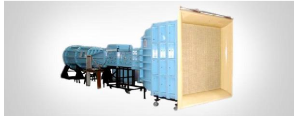
Figure 3 Wind tunnel used for smoke flow visualization
