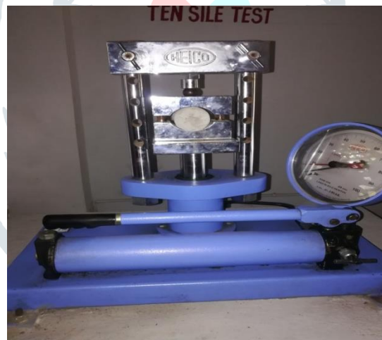
Fig. 5 Testing the rock sample with tensile test
