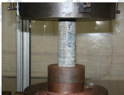
Fig 7: A sample under UCS test
