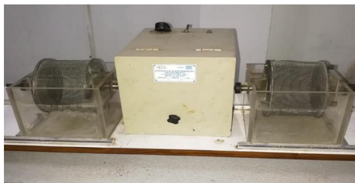
Fig. 2 Slake durability testing machine
