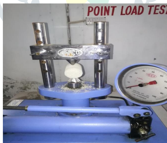
Fig. 3 Point load test for rock sample
