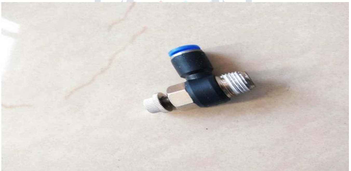
FLOW CONTROL VALVE
