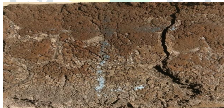
Figure 4: Modified brick sample showing the development of the shear plane in sample.
