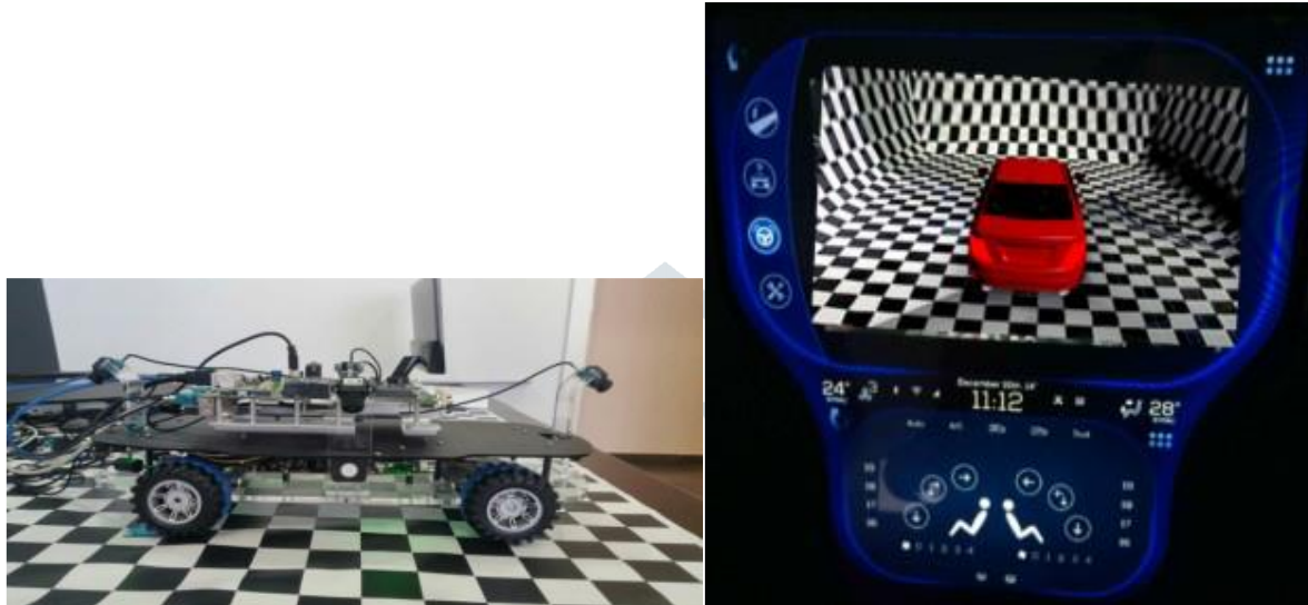
Figure 3: The surround view system prototype and bird eye view
