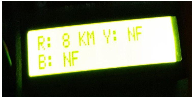
Figure 10 fault is created near 8km in R phase
