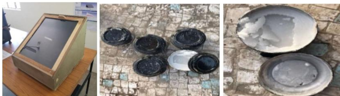
Figure 3 Actual Solar still and stearic acid containers as pcm material
