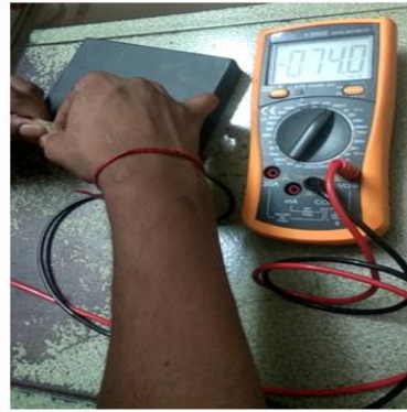
Fig 4b Output voltage of series 0.5% &amp; 1% Ga-ZnO/PVDF NG
