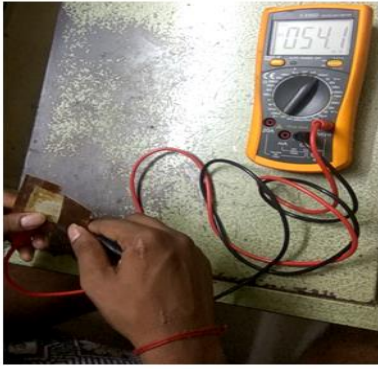
Fig 4a Output voltage of 2% Ga-ZnO/PVDF NG
