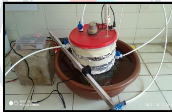
Fig 4: Hot water bath for anaerobic reactor
