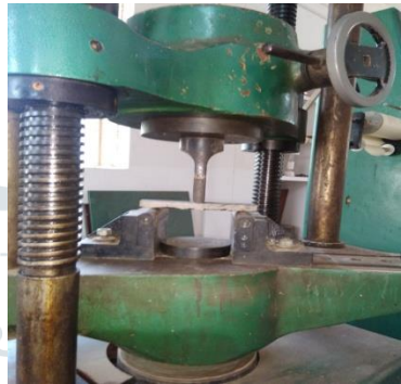
Fig. 3. Specimen under Flexural test
