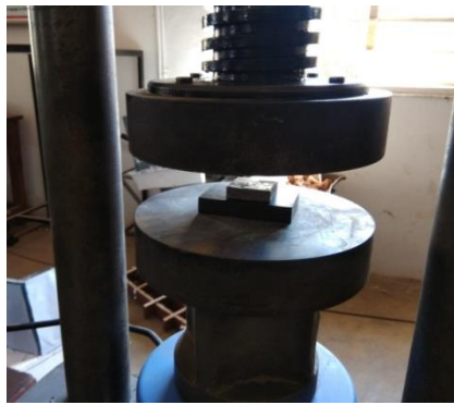
Fig. 5. Specimen under Compression test
