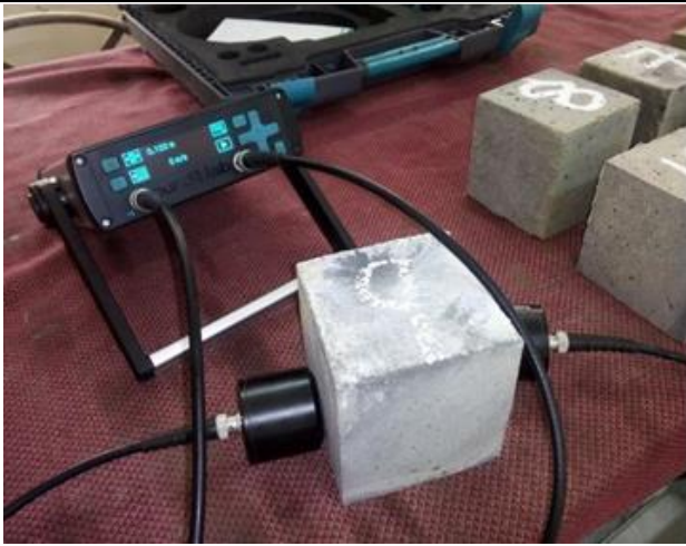
UPV test set up
