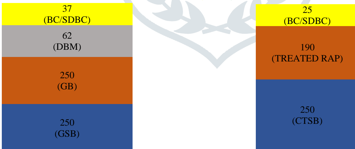
Figure 6: Pavement Composition of GB & GSB and RAP
