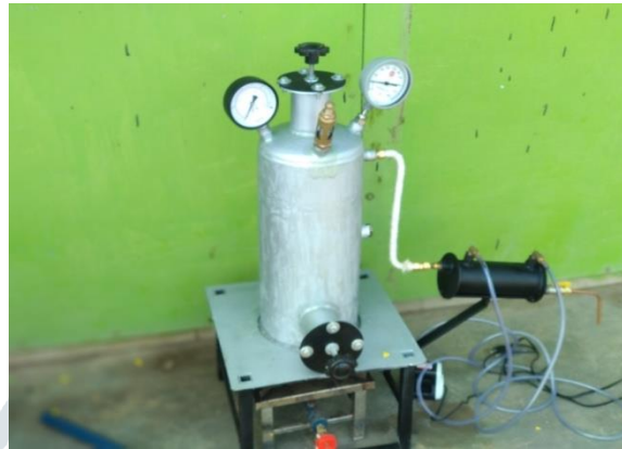
Fig 1.1: Experimental setup for Pyrolysis process
