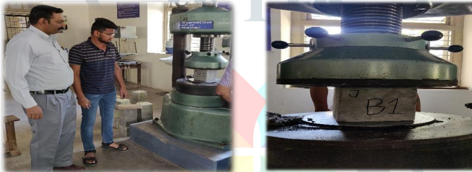
Figure 2 Setup of compressive strength testing of concrete specimen
