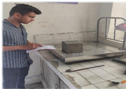
Figure 3 Water absorption test for concrete
