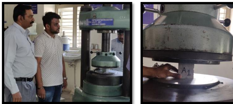
Figure 2 Setup of compressive strength testing of mortar
