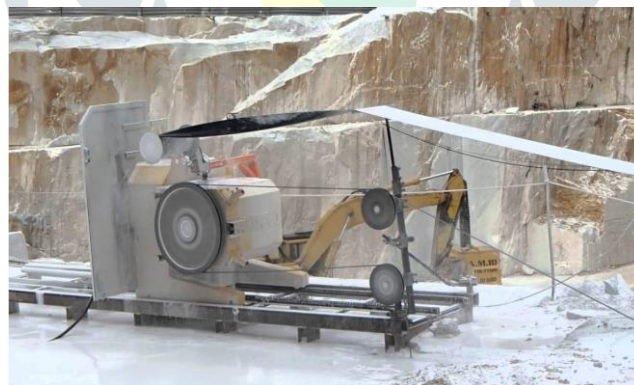
Fig.4 wire saw machine
