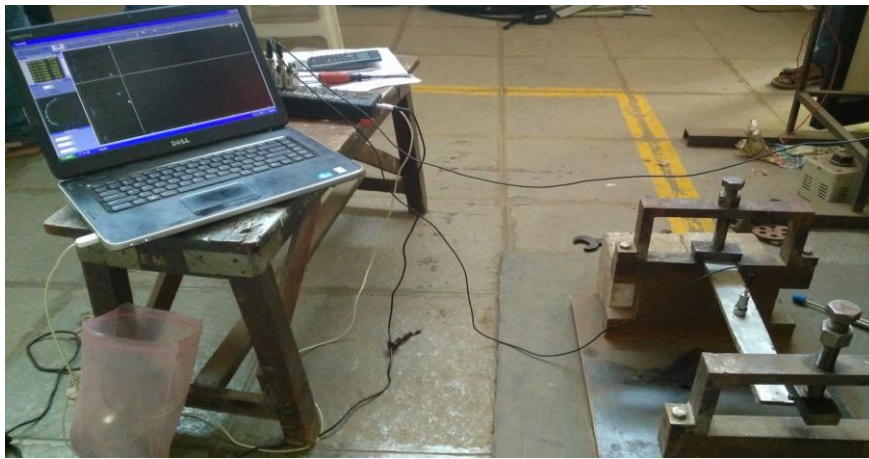
Fig 9: FFT Analyzer and Data Acquisition System for Impulse-Hammer Test
