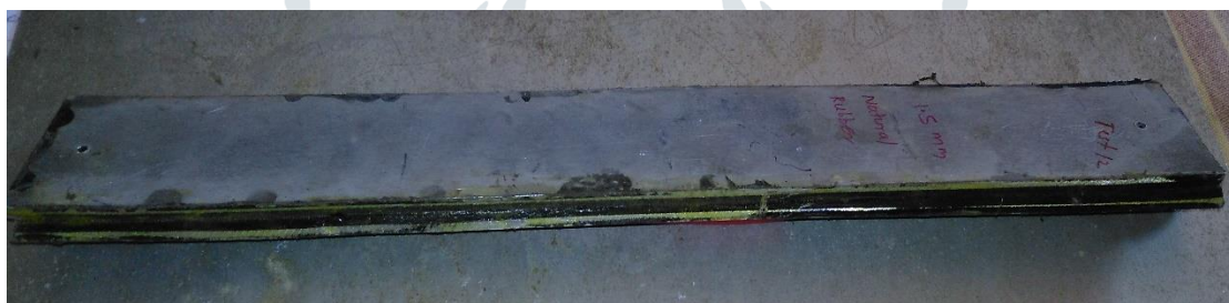
Fig.8: 3mm Natural Rubber coated Constrained layer Specimen
