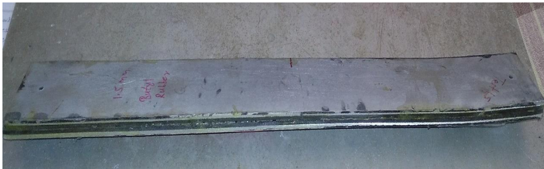
Fig.7: 3mm Butyl Rubber coated Constrained layer Specimen
