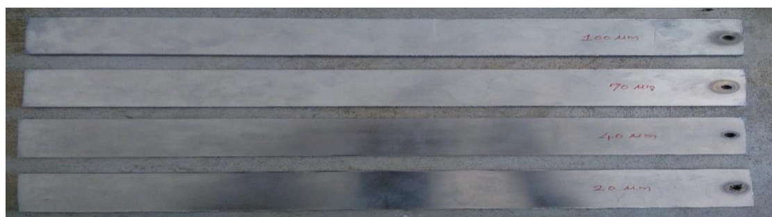
Fig.5: Specimens-01, 02, 03 and 04 - 20 μm, 40μm, 70μm and 100 μm Chrome Plated
