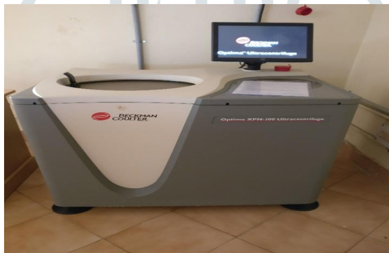
Fig.2. Beckman Coulter Ultracentrifuge equipment
