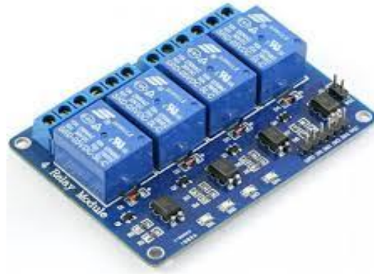
Fig.7 4 Channel 5V relay module with optocoupler isolation
