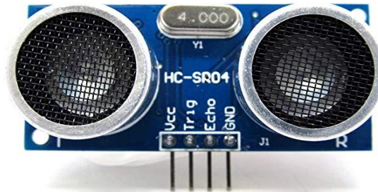
Fig.4 HC-SR04 ultrasonic level sensor
