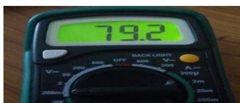
Figure 8- tested result 79 mV approx. one module (tested result)
