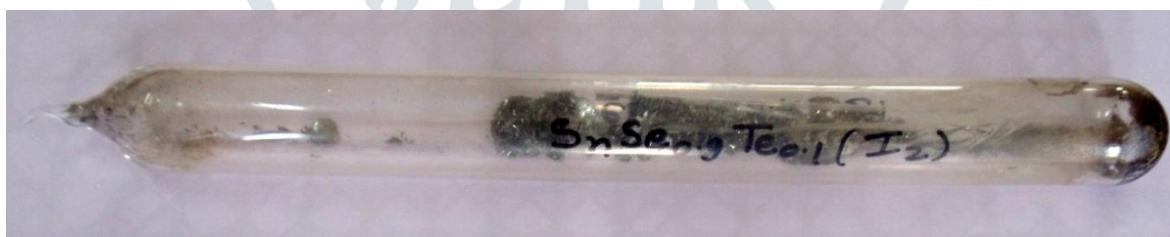
Figure.1 Crystals of \text{SnSe}_{0.9}\text{Te}_{0.1} ( \text{I}_2 ) inside the Quartz Ampoule.
