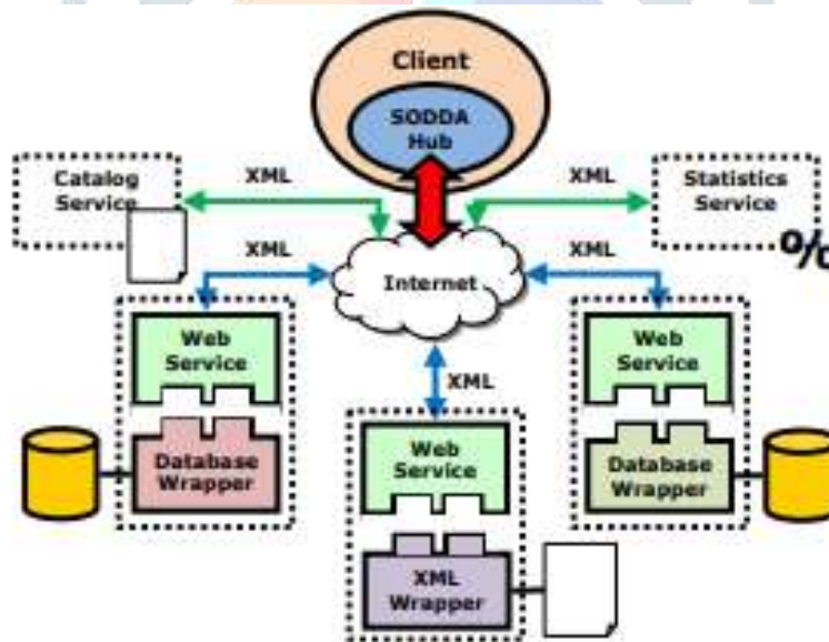
Figure 1: Basic layout of the service-oriented distributed database architecture
