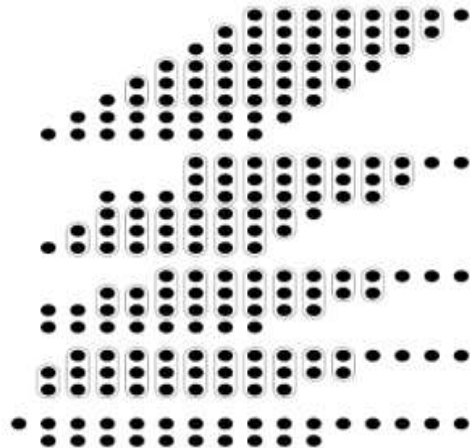
Fig. 4.1: Modified Wallace-Tree Multiplier
